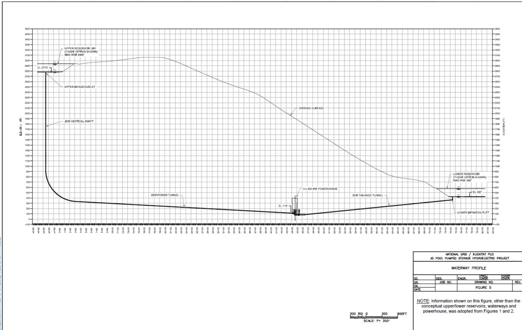
Figure 1.5-4: Goldendale Energy Storage Project General Arrangement—Typical Profile
